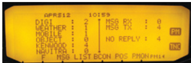
Figure 1 — This display shows how many beacons of each APRS “type” have been received.
