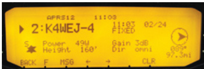
Figure 2 — Pressing the DETAIL button scrolls through screens of information available for each APRS station received. This screen shows information from a digipeater — power, height and antenna info.
