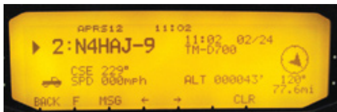
Figure 3 — Here's info on a mobile in motion (though his speed is zero, so he's sitting still). It shows the direction he's headed (229°), his altitude (43 feet) and that he's 77.6 miles southeast of me (the arrow pointing to 120°).
