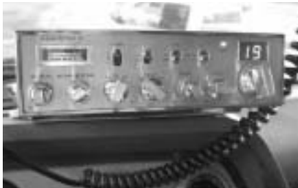
Channel 19 on this Connex 4400 "Export" radio, sitting on Derek's dash, can be one of 8 actual radio frequencies. One of them is 28.085 in the 10 meter band
