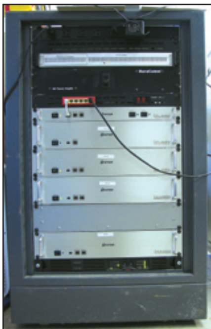
Figure 2 — The full stack of D-STAR equipment at the test bench of Jim McClellan, N5MIJ. From top to bottom, an IP-RP2C controller, an ID-RP2D 1.2 GHz data repeater, an ID-RP2V 1.2 GHz voice repeater, an ID-RP4000 440 MHz voice and data repeater, a blank panel and an ID-RP2000 146 MHz voice and data repeater.
